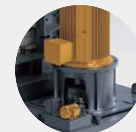
Drive System Equipped with fluid coupling to improve performance and reduce current during start-up. Optional VFD device for machine rotating speed control
